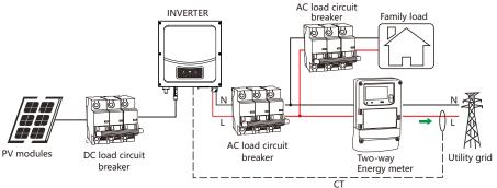
Note: Only for inverters with load matching functions, General PV grid inverter electrical installation diagram, please refer to the user manual.
