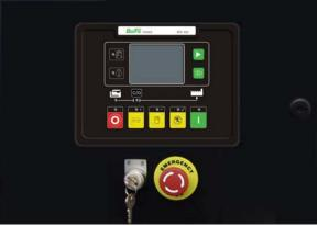
**Standard** Control **Panel** uses micro processing technique integrating digital, intelligent and network techniques which can carry out functions including auto start/stop, data measure, alarming. The controller uses LCD display, optional English display interface with operation easy and reliable. It can be widely used in all types of generator automatic control system for compact structure, advanced circuits, simple connections and high reliability
